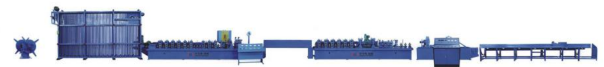
Uncoiler ▶ Pre-forming ▶ High frequency welder ▶ Post-forming ▶ Cutting to length ▶ Stake device
